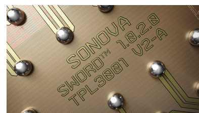
In 2018, we introduced our first products based on the proprietary SWORD™ (Sonova Wireless One Radio Digital) chip, an ultra-low power chip.
